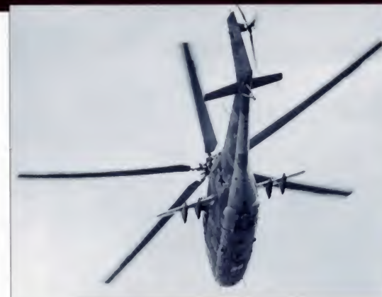
Straight wings without anhedral identify this Mi-24 as a 'Hind-B' from the first production series.
